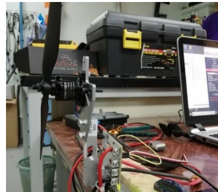
Figure 3: Thrust test conducted on 980KV motors
