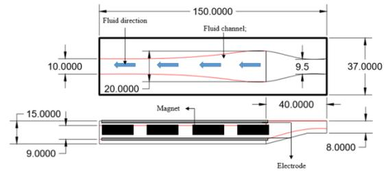
**Figure 4:** Magneto-hydrodynamic propulsion design
