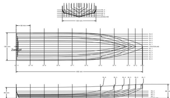
Figure 2: Lines plan of the boat model
