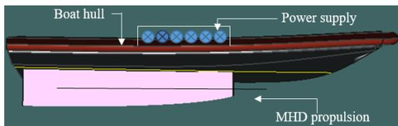
**Figure 3:** MHD propulsion boat model system arrangement
