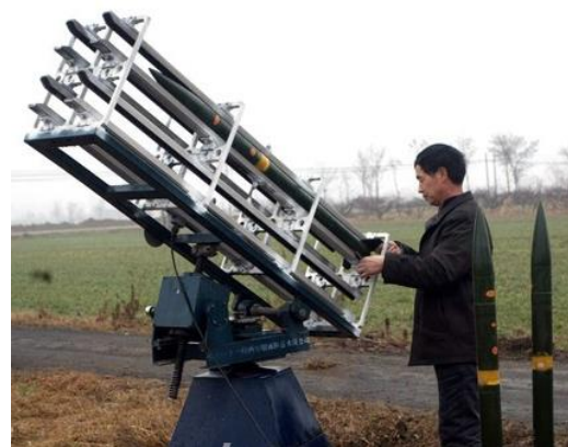
Figure 2: Cloud seeding process using rocket mechanism [17]
