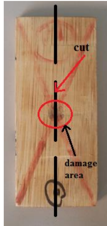
Figure 4: Preparation of specimen microscopic scan
