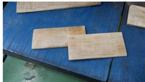
Figure 2: Flat plate specimen of pure bamboo
