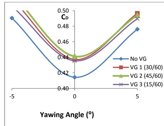
Figure 9: Close-up view of Figure 8 (Yaw Angle -5o to 5o)
