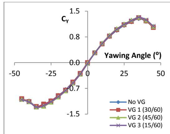
Figure 12: Comparison of Side Force Coefficient at Various VGs
