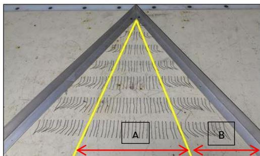
Figure 15: Flow Reattachment Line with VG 1 (30/60)
