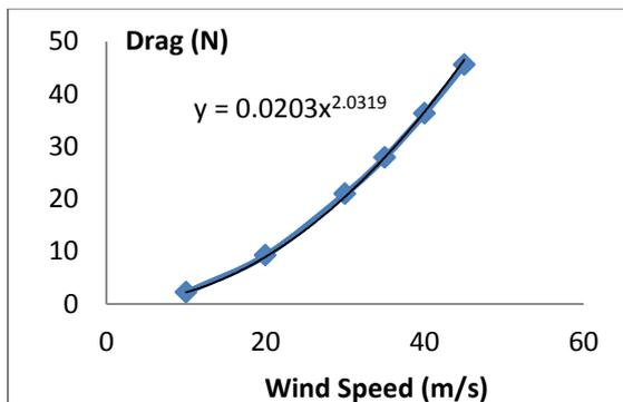
Figure 7: The graph of Drag vs Wind Speed
