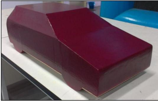
Figure 3: The simplified Hyundai Veloster wind tunnel model
