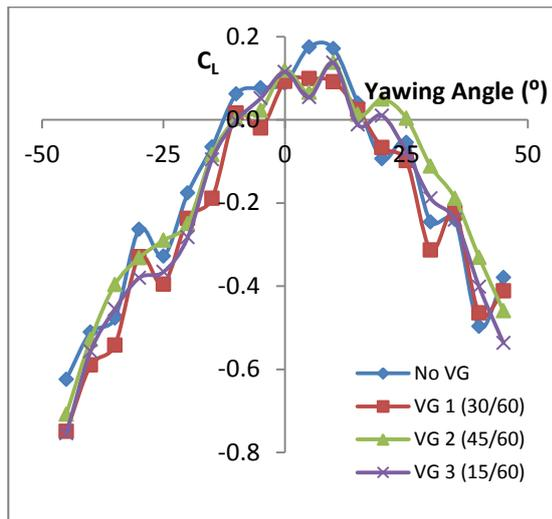
Figure 14: Comparison of Lift Coefficient at Various VGs
