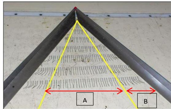
Figure 17: Flow Reattachment Line with VG 3 (15/60)
