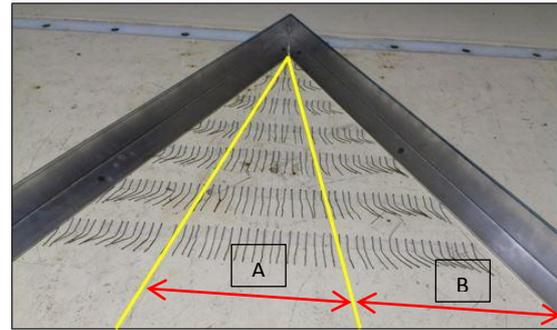
Figure 16: Flow Reattachment Line with VG 2 (45/60)
