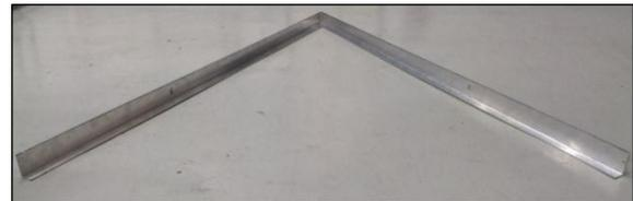
Figure 1: Vortex Generator 2 (45mm/60mm)
