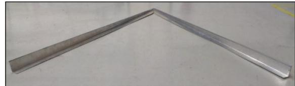
Figure 2: Vortex Generator 3 (15mm/60mm)
