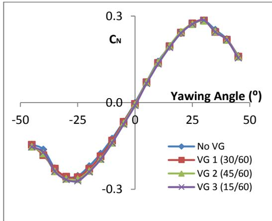
Figure 10: Comparison of CN at Various VGs
