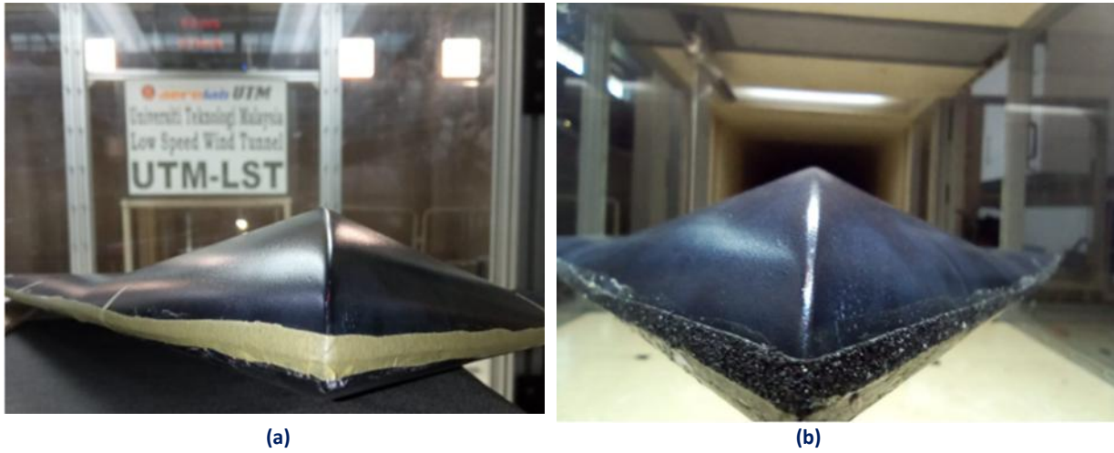
Figure 5: Summary of the transition strips applied to the MULDICON wing: (a) 2D adhesive transition strip at the leading edge and (b) 3D carborundum-grit transition strip at the leading edge.
