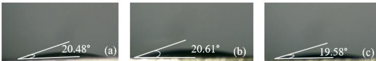
Figure 3: Contact angle of PAO4 with GMO 7wt% on the steel surface in temperatures (a) 25°C, (b) 40°C, and (c) 60°C
