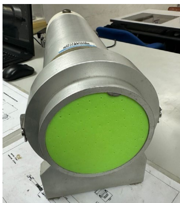
Figure 7: MPP installed in front of the flat rigid wall back
