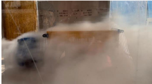
Figure 12: Lorry with Cylinder Positions 2B and 5 during testing [21]
