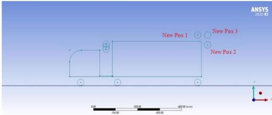
Figure 1: Geometric Model of Lorry with Three New Positions of Cylinder [19]
