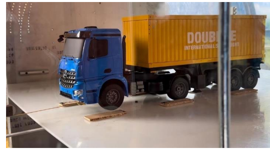
Figure 7: Lifting of Lorry (Baseline Condition) during testing [21]
