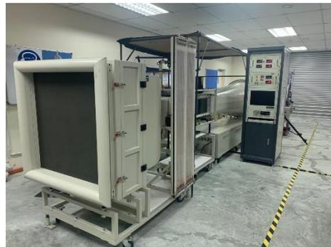
**Figure 6:** Longwin LW-9300R wind tunnel
