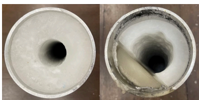
Pure paraffin wax before (left) and after (right) burning.
