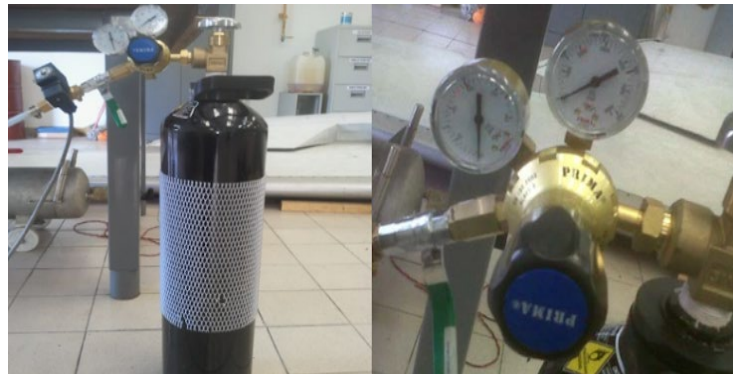
Figure 6: Oxygen gas that has been pressurised (left) and a gas regulator (right)
