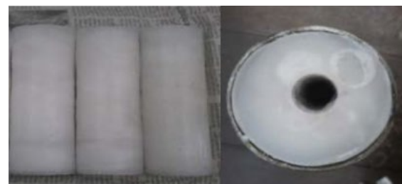
Figure 4: Paraffin fuel that has been moulded
