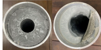
PW+Al 1% before (left) and after (right) burning.
